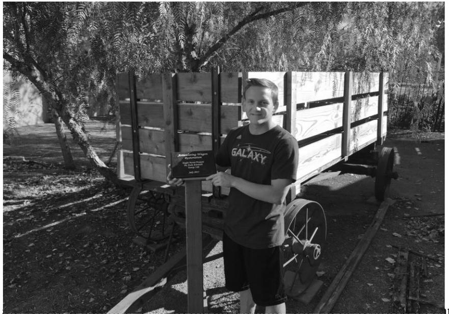
Rare Kitchell standing next to the amazing wagon he restored as part of his Eagle Scout project requirement. The unique thing about this type of wagon is that when the towing tongue is turned the rear wheels turn in the opposite direction allowing for tight turns at the end of rows of crops.
